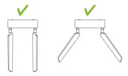
Warning: Incorrect antenna positioning can affect antenna performance.
