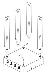
2. Attach the cable assembly to the 4 SMA connectors on the side of the Extended Antenna Mount (Part A). Ensure the labels on the cable match the labels on the connector.
