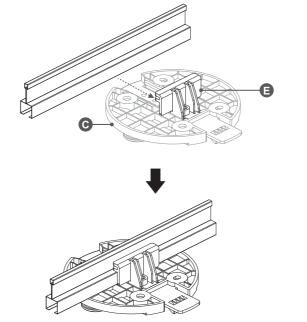
5. Secure the other hook (Part E) onto the Mounting Bracket (Part C) using screws (Part D) to ensure a tight fit. Slide the other hook in place to ensure a tight fight on the rail. Secure in place by tightening the provided screw as illustrated below.
