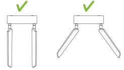
Warning: Incorrect antenna positioning can affect antenna performance.
