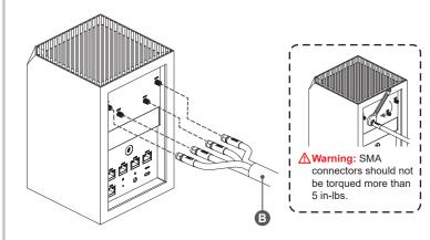
Position the antennas as illustrated below. Ensure the Mount is firmly secured on the ceiling through screw.
