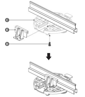
Combine the Extended Antenna Mount (Part A) to the bracket (Part C) on the rail, and slide it towards the bracket latch until you hear a clicking sound.
