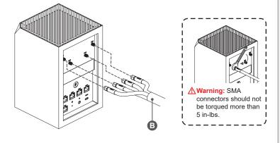
Position the antennas as illustrated below. Ensure the Mount is firmly secured on the rail through screw.
