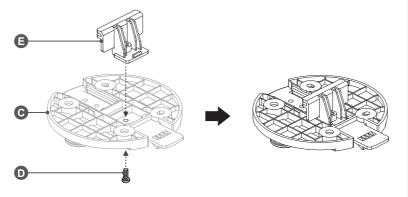
Place the Mounting Bracket (Part C) on one side of the rail as illustrated below.
